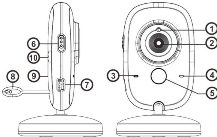
1. **Light sensor** - Allows the baby unit to correct itself under changing light conditions.
