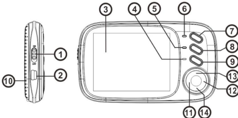
1. **On/Off button** - Turns the parent unit ON or OFF.
